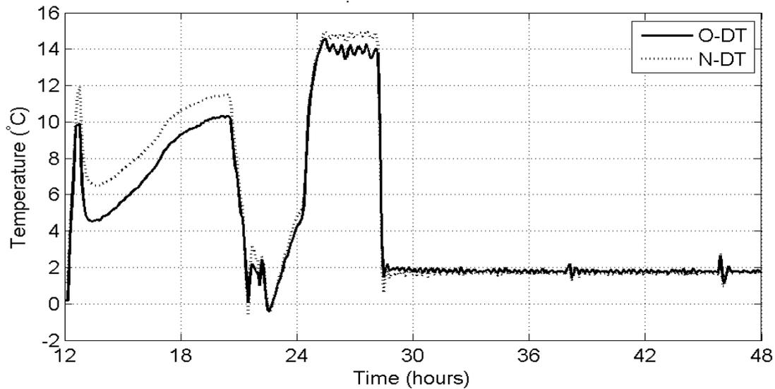
**Figure 17. Mean surface temperature for the original (O) and the new (N) EPS boxes during a dynamic temperature period. The mean surface temperature was calculated from the top and second top boxes for each group.**
