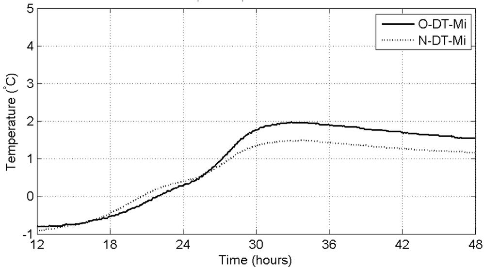
**Figure 19.** Mean product temperature in the middle of the original (O) and the new (N) EPS boxes during a dynamic temperature period. The mean product temperature was calculated from four middle positions in the top and second top boxes for both the original and the new boxes.
