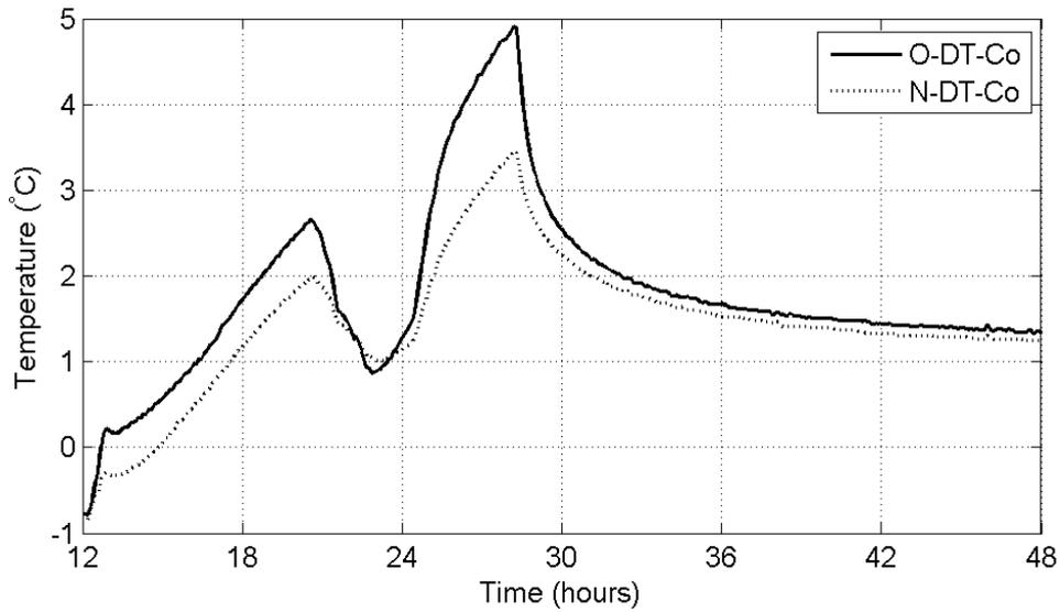
**Figure 18.** Mean product temperature at the bottom corners of the original (O) and the new (N) EPS boxes during a dynamic temperature period. The mean product temperature was calculated from four bottom corner positions in the top and second top boxes for both the original and the new boxes.
