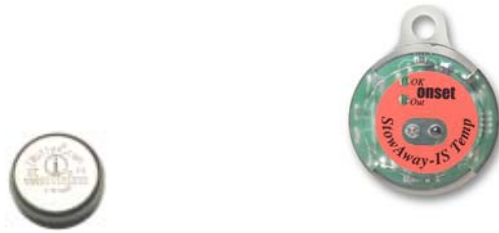
Figure 3: Temperature loggers used in the study. iButton loggers with 17 mm diameter and 6 mm thickness (left) and Onset Stowaway loggers with 38 mm diameter and 20 mm thickness (right).
