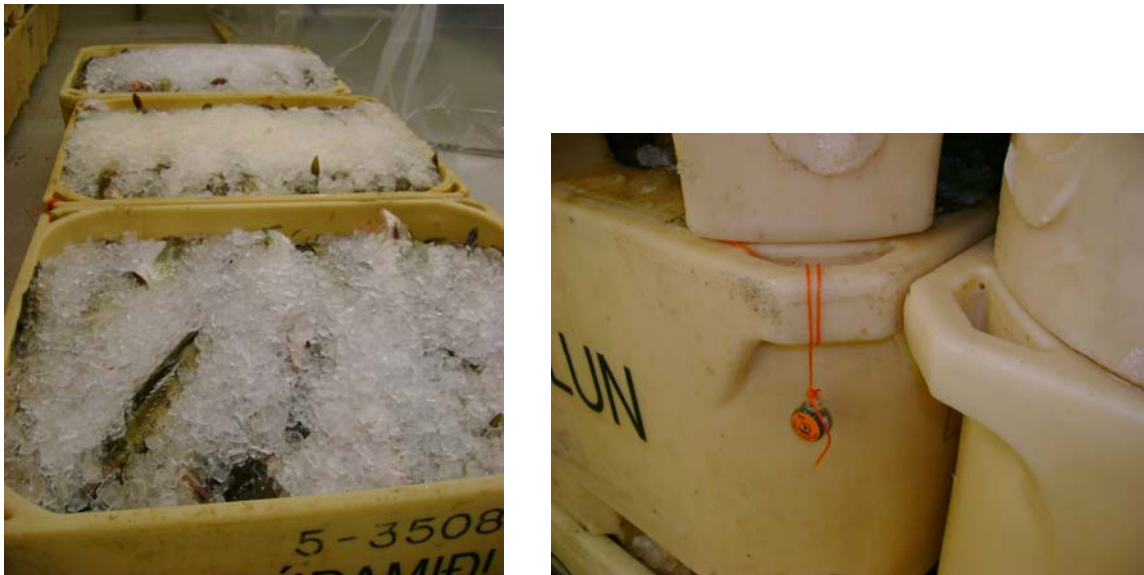
Figure 1: Whole, bled and gutted cod ( Gadus morhua ) iced in 460 L plastic tubs (left). Temperature loggers for ambient temperature measurements tied to tubs (right).
